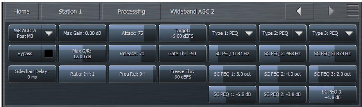
The **Wideband AGC2** menu provides access to the transient enhance, maximum gain, maximum gain reduction, ratio, attack, release, progressive release, target, gate threshold, freeze threshold, and three-band sidechain parametric equalizer controls.
