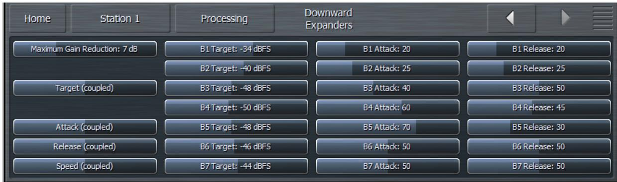
The Downward Expanders operates in a manner similar to a traditional “noise gate,” and is useful for reducing unwanted background noise from less-than-perfect program material or from a noisy studio environment. The ratio of these expanders is 2:1.
